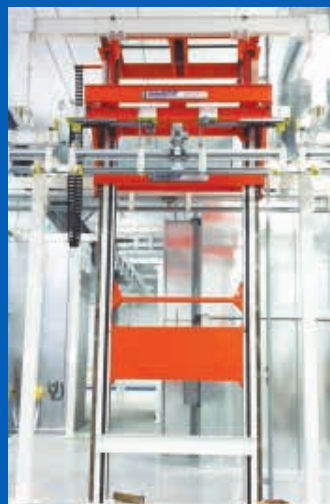
Vertical lifts used for larger elevation changes.
